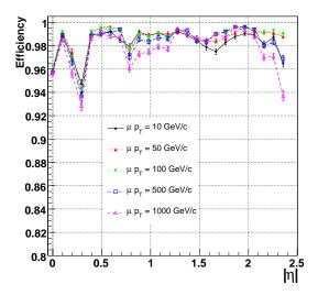
Figure 134: Muon reconstruction efficiency as a function of pseudorapidity for selected values of  $p_T$ . Left panel: standalone reconstruction (using only hits from the muon system with a vertex constraint). Right panel: global reconstruction (using hits from both the muon system and the tracker).
