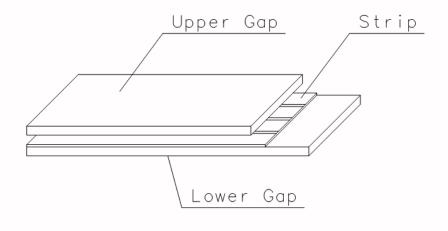
Figure 198: Layout of a double-gap RPC.
