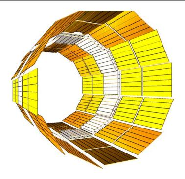
Figure 114: Layout of all the HO trays in the CMS detector.
