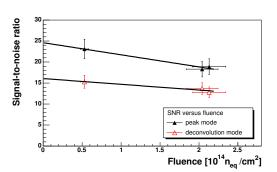
Figure 70: Signal-to-noise ratio versus fluence for modules with  $500 \,\mu\text{m}$  (left panel) and  $320 \,\mu\text{m}$  thick sensors (right panel) in peak (filled symbols) and deconvolution mode (open symbols).
