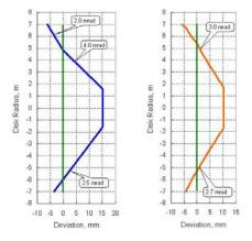
Figure 225: Comparison of the YE+1 disk deformations in the r-z plane at full magnetic field (4 T) measured by the alignment system (left panel) and predictions from finite element analysis (right panel). The vertical lines correspond to 0 magnetic field.
