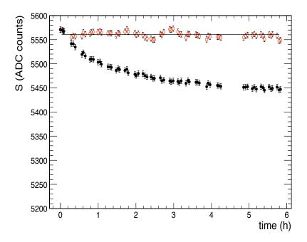
Figure 89: Effect of the monitor correction procedure on test beam data: full black points refer to signals measured during test beam irradiation, open red points are the same after the monitor corrections.
