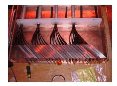
Figure 131: The side view of the ZDC showing the EM and HAD sections.
