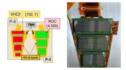
Figure 46: Sketches of the two types of FPix panels showing the different sizes and numbers of the plaquettes on each (left side). A photograph of an actual 3-plaquette panel (right side).
