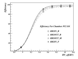
Figure 217: Global efficiency vs.  $HV_{\rm eff}$ , estimated by means of DT segment extrapolation.
