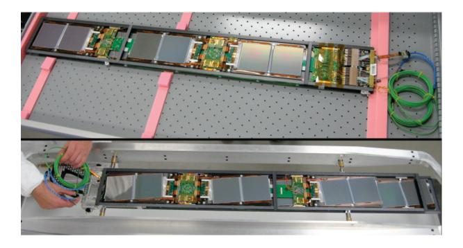
Figure 57: Top panel: photo of an assembled double-sided rod, showing the CCUM side, with the 12-way optical ribbons connected to the AOH fibers. Bottom panel: double-sided rod being prepared for insertion in the TOB mechanics; the side opposite to the CCUM is shown.
