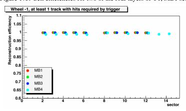
Figure 174: Reconstruction efficiency with 7 points in both  $\Phi$ -type superlayers, according to the trigger condition, requiring either two 4-hit segments in both of the two  $\Phi$ -type superlayers or one 4-hit and one 3-hit segment.
