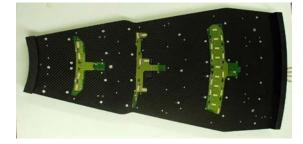
Figure 61: The different ICBs on the two sides of a front petal: ICB\_2 and ICB\_46 on side B, and ICB\_1, ICB\_3 and ICB\_57 on side A (from left to right). On ICB\_46, the two CCUMs are plugged.
