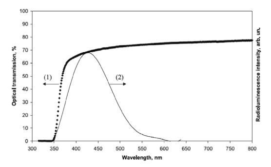
Figure 71: Longitudinal optical transmission (1, left scale) and radioluminescence intensity (2, right scale) for production PbWO<sub>4</sub> crystals.
