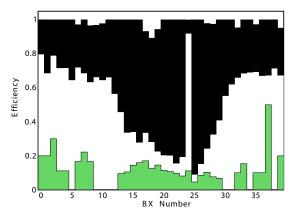
Figure 170: Distribution of the BX assigned to the tracks found by the PHTF. The BX is correctly identified when its value is 24. Superimposed are the distributions of the same quantity determined independently by the local trigger in MB1 and MB3, as well as the distribution of the determined BX when a trigger segment at the same BX was delivered in coincidence in MB1 and MB3.
