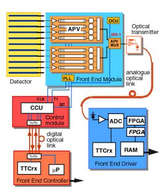
Figure 49: Read-out scheme of the CMS tracker.
