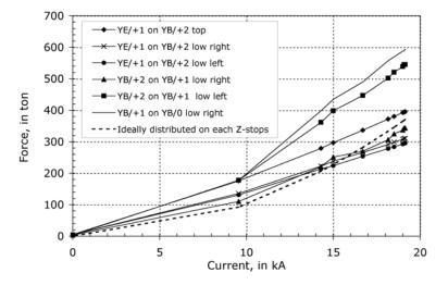
Figure 26: Axial forces acting on the yoke Z-stops during the coil energising.
