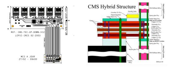
Figure 50: Front-end hybrid layout (example for TEC shown on the left) and arrangement of layers.
