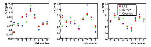
Figure 64: TEC+ disk rotation  $\Delta \phi$  (around the beam axis) and displacements  $\Delta x, \Delta y$  (in the disk plane) as determined from survey, LAS and cosmic muon tracks.
