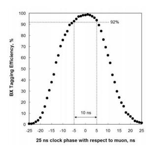
Figure 193: Left panel: Time distributions of the response of a single plane to a passing muon (top) and for the 3rd earliest hit in an ALCT pattern (bottom). The horizontal scale has an arbitrary offset. The shaded band indicates the 25-ns window, the time between bunch crossings at the LHC. Right panel: Probability for correct bunch-crossing tagging vs. relative phase shift between the 25-ns clock on an ALCT board and the LHC 25-ns clock.
