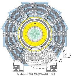
Figure 175: The MTCC exploited in the barrel region three sectors in wheels YB+1 (sector 10) and YB+2 (sectors 10, 11) instrumented with DTs and RPCs.
