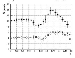
Figure 31: Number of measurement points in the strip tracker as a function of pseudorapidity  $\eta$ . Filled circles show the total number (back-to-back modules count as one) while open squares show the number of stereo layers.
