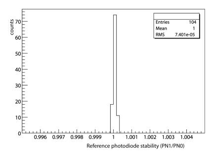
Figure 87: Relative stability between a pair of reference PN photodiodes monitoring 200 crystals measured in autumn 2004 at the CERN test beam facility.
