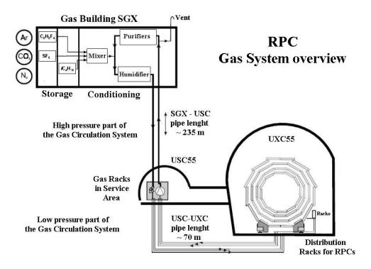
Figure 207: Closed-loop circulation system.
