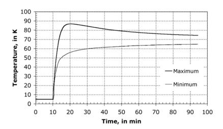
Figure 23: Minimum and maximum temperatures detected on the cold mass during the fast discharge from  $19.1 \, \mathrm{kA}$ .
