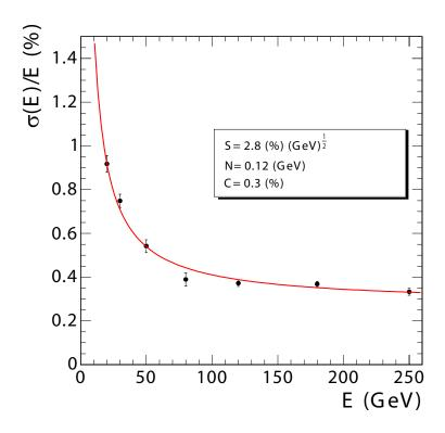
Figure 3: ECAL energy resolution,  $\sigma(E)/E$ , as a function of electron energy as measured from a beam test. The energy was measured in an array of  $3 \times 3$  crystals with an electron impacting the central crystal. The points correspond to events taken restricting the incident beam to a narrow  $(4 \times 4 \text{ mm}^2)$  region. The stochastic (S), noise (N), and constant (C) terms are given.
