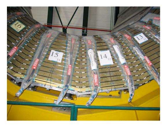
Figure 99: Close up view of the assembled HB wedges, showing the optical cabling.
