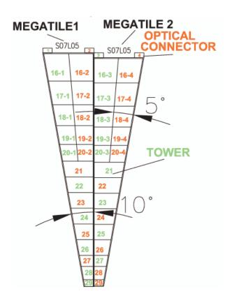
Figure 107: Numbering scheme for the tiles in adjacent scintillator trays.
