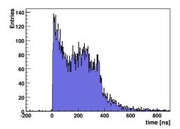
Figure 151: Drift Time distribution of a good cell. Wire position corresponds to time 0.
