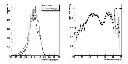
Figure 177: Left panel: Distribution of  $t_0$  for all track segments in a station, for events triggered by RPC (solid line). The distribution of the same quantity for events also triggered by the DT is superimposed (dashed line). Right panel: DT local trigger efficiency as a function of the quantity  $t_0$ , obtained by the ratio of the two histograms shown on the left.
