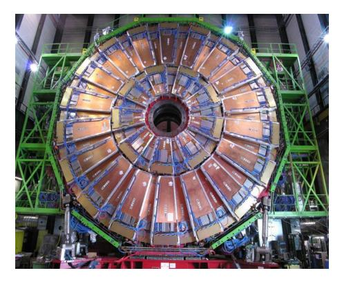
Figure 180: The ME2 station of CSCs. The outer ring consists of 36 ME2/2 chambers, each spanning  $10^{\circ}$  in  $\phi$ , and the inner ring of eighteen  $20^{\circ}$  ME2/1 chambers. The chambers overlap to provide contiguous coverage in  $\phi$ .
