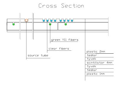
Figure 97: Cross-sectional view of a scintillator tray.
