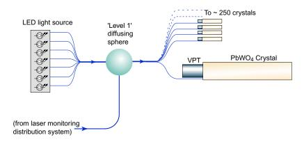
Figure 78: Distribution system for VPT stabilisation light pulses.
