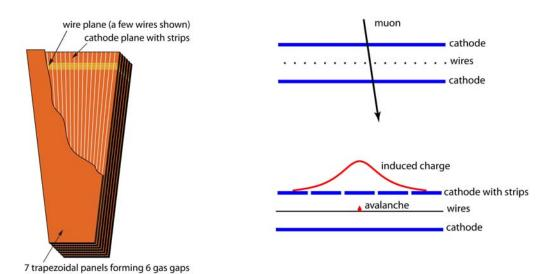
Figure 181: Layout of a CSC made of 7 trapezoidal panels. The panels form 6 gas gaps withplanes of sensitive anode wires. The cut-out in the top panel reveals anode wires and cathode strips. Only a few wires are shown to indicate their azimuthal direction. Strips of constant  $\Delta\phi$  run lengthwise (radially). The 144 largest CSCs are 3.4 m long along the strip direction and up to 1.5 m wide along the wire direction.
