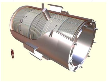
Figure 5: General artistic view of the 5 modules composing the cold mass inside the cryostat, with details of the supporting system (vertical, radial and longitudinal tie rods).
