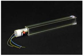
Figure 72: PbWO4 crystals with photodetectors attached. Left panel: A barrel crystal with the upper face depolished and the APD capsule. In the insert, a capsule with the two APDs. Right panel: An endcap crystal and VPT.
