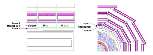
Figure 110: Longitudinal and transverse views of the CMS detector showing the position of HO layers.
