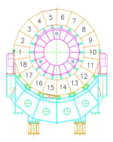
Figure 94: Numbering scheme for the HB wedges. Wedge 1 is on the inside (+x direction) of the LHC ring.
