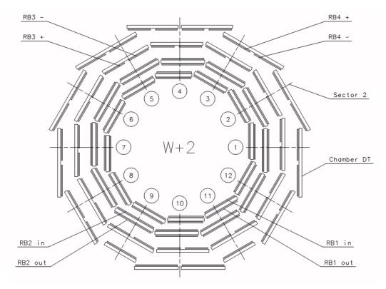
Figure 199: Schematic layout of one of the 5 barrel wheels, which are labeled -2, -1, 0, +1, and +2, respectively. Each wheel is divided into 12 sectors that are numbered as shown.
