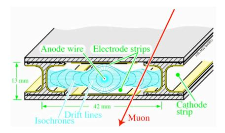
Figure 137: Sketch of a cell showing drift lines and isochrones. The plates at the top and bottom of the cell are at ground potential. The voltages applied to the electrodes are +3600V for wires, +1800V for strips, and -1200V for cathodes.
