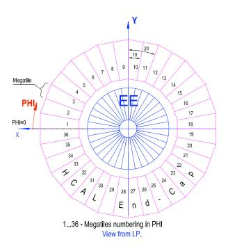
Figure 108: Numbering scheme for the HE wedges as viewed from the interaction point. The +x direction points to the center of the LHC ring.
