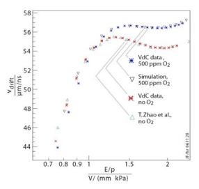
Figure 140: Calculated drift velocity (in cm/ $\mu$ s) as a function of the electric field (in V/cm) for a gas mixture Ar/CO<sub>2</sub> (85%/15%). The values obtained are very similar for the 2 different environment pressures, 973 and 1027 hPa.
