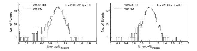
Figure 112: A simulation of the distribution of the measured energy scaled to the incident energy for pions with incident energies of (left panel) 200 GeV at  $\eta = 0$  and (right panel) 225 GeV at  $|\eta| = 0.5$ . The solid and dashed histograms are measurements without and with HO, respectively.
