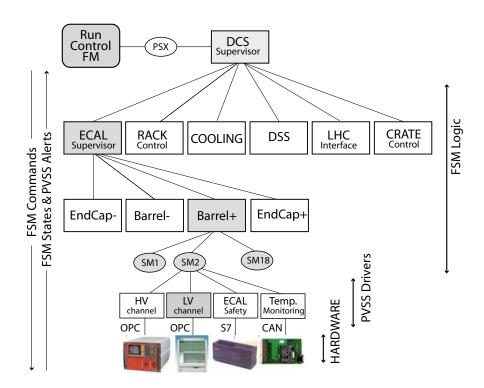
Figure 249: Outline of the Detector Control System hierarchy. Shown are all global services and ECAL as an example of a sub-detector control.
