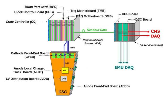
Figure 186: Schematic layout of the CSC trigger and read-out electronics.
