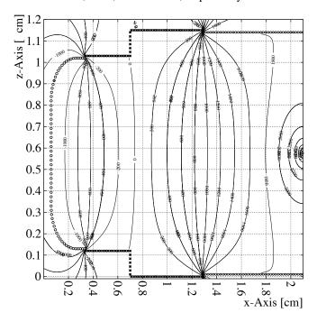
Figure 142: Equipotential lines in half of a drift cell. The anode wire is on the right side. The lines are labeled with the potentials in volts (the x-axis is perpendicular to the wire on the wire plane, while the z-axis is orthogonal to the wire plane).
