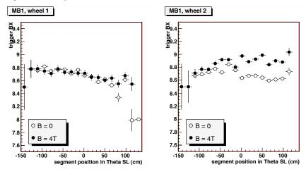
Figure 178: BX determined by the DTLT as a function of the track position in the z-direction of the muon station, with and without magnetic field, for MB1 in Wheel 1 on the left, where no effect of the B-field is expected. On the right, the same quantities are shown for MB1 in Wheel 2, where an influence of the magnetic field on the drift velocity is expected.
