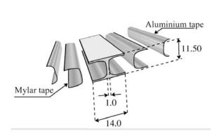
Figure 138: Exploded view of the cathode electrodes, glued on the I-beams.
