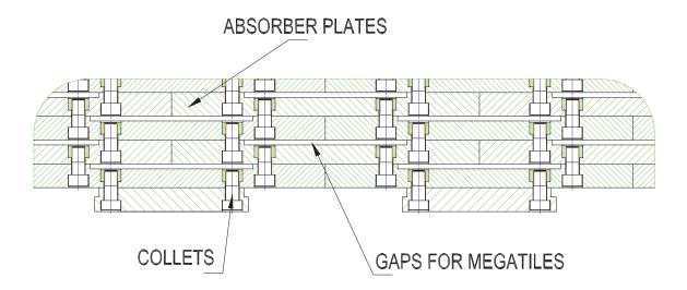
Figure 104: Mechanical structure of the HE absorber. Particles enter the calorimeter from the bottom.
