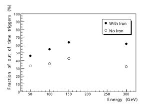
Figure 168: Fraction of ghost triggers observed in a muon station in single muon events, defined as the ratio of the number of second tracks over the number of first tracks, delivered by the local trigger at the correct BX, as a function of the muon momentum, for events with and without the iron absorber.
