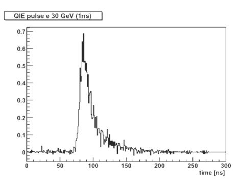
Figure 125: Measured single event pulse shape from the scintillator tiles, representative of HB/HE/HO pulse shapes.
