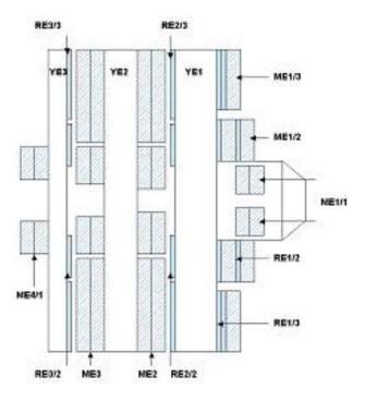
Figure 203: Schematic layout of the CMS endcap for the initial muon system.
