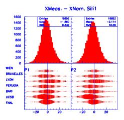
Figure 52: A typical residual distribution (in  $\mu$ m) for a reference point on the modules is shown for the different module assembly centers, indicating a precision of 10  $\mu$ m (RMS) in the module production.
