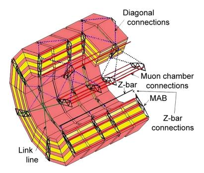
Figure 219: Schematic view of the barrel monitoring system showing the optical network among the MAB structures.
