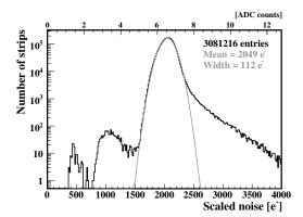
Figure 66: Normalized common mode subtracted noise of all strips (scaled to the strip length of ring 1 sensors) of both TECs (left panel) and the TOB (right panel), in deconvolution mode. Details are described in the text.
