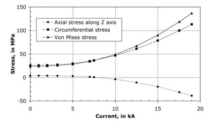
Figure 20: Stresses measured on the CB0 module as a function of the current.
