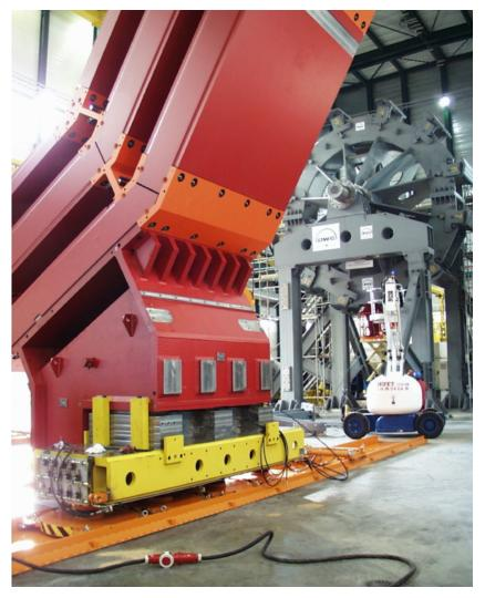
Figure 252: A transport beam for barrel rings with 4 air pads fixed on it.
