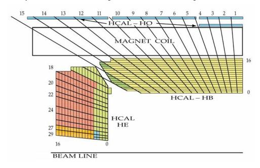
Figure 101: The HCAL tower segmentation in the r, z plane for one-fourth of the HB, HO, and HE detectors. The shading represents the optical grouping of scintillator layers into different longitudinal readouts.
