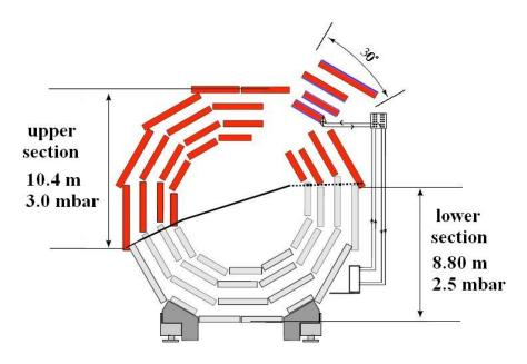
Figure 208: The 2 zones into which a wheel is sub-divided. Each station (2 chambers) is supplied by a gas line.
