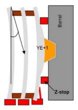
Figure 226: Current understanding of disk deformation due to magnetic forces based on alignment system measurements. The z-stops (red) prevent the disks from getting pushed into each other. Note that the indicated bending angle is exaggerated for illustrative purposes. Its measured magnitude is 2.5 mrad.
