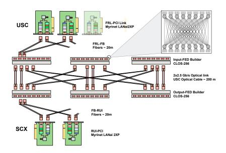
Figure 244: The FED builder stage switching fabric (only 1 rail is shown).
