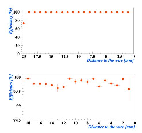
Figure 161: Efficiency as a function of the distance to the wire (top), for tracks orthogonal to chamber surface; (bottom) with an expanded scale excluding the I-beam region.
