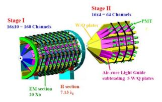
Figure 130: Details of the components and geometry of the CASTOR calorimeter.
