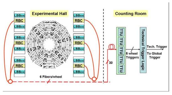
Figure 206: Technical Trigger schematic layout.
