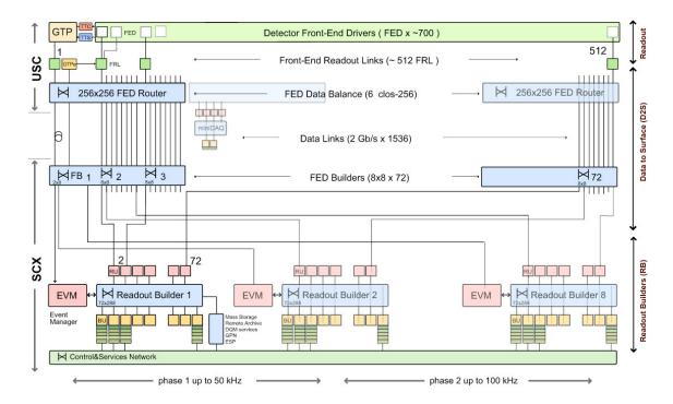
Figure 242: Schematic view of the Event Builder.
