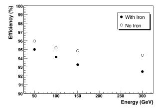
Figure 167: BX identification efficiency in a muon station in single muon events, as a function of the incident muon momentum, for events with and without the iron absorber placed in front of the muon station.
