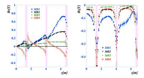
Figure 164: Radial ( $B_r$ ) and longitudinal ( $B_z$ ) components of the CMS magnetic field in the regions where the barrel chambers are placed as a function of the position along the beam direction (the centre of the detector is at z=0). Vertical bands indicate the separation between chamber wheels (in these particular regions  $B_z$  becomes significant). The biggest  $B_r$  values (0.7–0.8 T) occur in the MB1 region near the endcaps.
