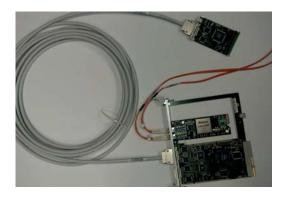
Figure 238: Photograph of S-link64 sender card, LVDS cable and compact-PCI FRL card with embedded LANai2XP NIC. Connected to the NIC are fibres that go to the FED Builder input switch.
