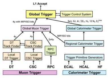
Figure 227: Architecture of the Level-1 Trigger.
