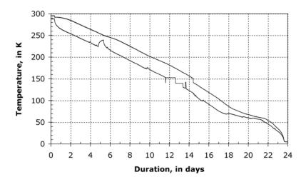
Figure 13: Graph of the coil minimum and maximum temperatures during the cool-down from room temperature to 4.5 K.
