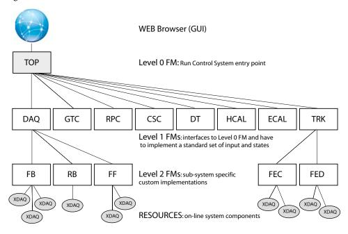
Figure 248: The RC hierarchy showing the full DAQ system. The Top Function Manager controls the next layer (Level 1) of Function Managers who in turn control the Level 2 (sub-detector level) Function Managers. The sub-detector Function Managers are responsible for managing the online system component resources.
