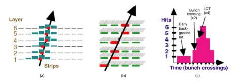
Figure 231: Cathode Strip Chamber Local Trigger: (a) Cathode LCT formation from strips, (b) Anode LCT formation from wire group hits, (c) Bunch crossing assignment.
