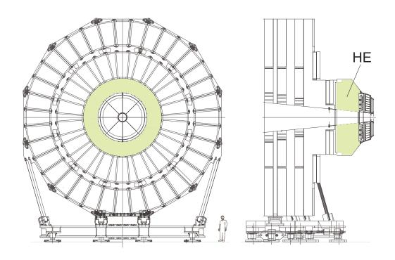
Figure 102: Hadron endcap (HE) calorimeter mounted on the endcap iron yoke.
