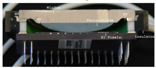
Figure 100: Cross sectional view of an HPD.
