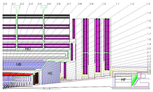
Figure 92: Longitudinal view of the CMS detector showing the locations of the hadron barrel (HB), endcap (HE), outer (HO) and forward (HF) calorimeters.
