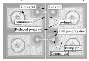
Figure 37: Photograph of four pixel cells. The Indium bumps are already deposited but not yet reflown.
