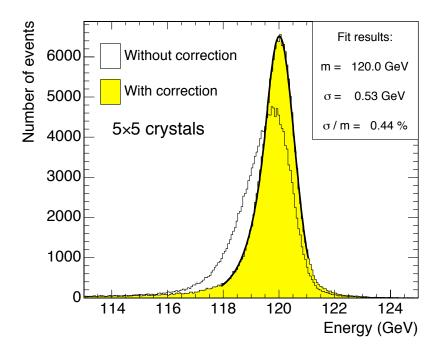
Figure 91: Distribution of energy reconstructed in a  $5 \times 5$  matrix, before and after correction for containment, when 120 GeV electrons are incident over a  $20 \times 20 \text{mm}^2$  area.
