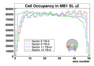
Figure 172: Sum of the occupancy of the four layers in MB1  $\Phi$ 1 superlayer for sectors 8, 9, 11 and 12. The sectors have different inclinations as shown on the right. Material inside the yoke along with the iron yoke itself shield partly the soft cosmic ray muons.
