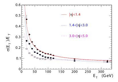
Figure 4: The jet transverse-energy resolution as a function of the simulated jet transverse energy for barrel jets ( $|\eta| < 1.4$ ), endcap jets ( $1.4 < |\eta| < 3.0$ ), and very forward jets ( $3.0 < |\eta| < 5.0$ ). The jets are reconstructed with an iterative cone algorithm (cone radius = 0.5).
