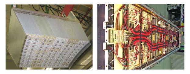
Figure 74: Left panel: front view of a module equipped with the crystals. Right panel: rear view of a supermodule, with the electronics, services and cables mounted.
