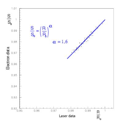
Figure 85: Relation between the transmission losses for scintillation light and for laser light for a given crystal. The signals are followed during the irradiation and the recovery.
