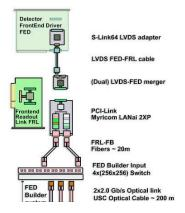
Figure 237: Diagram of a generic sub-detector readout into the FED builder.
