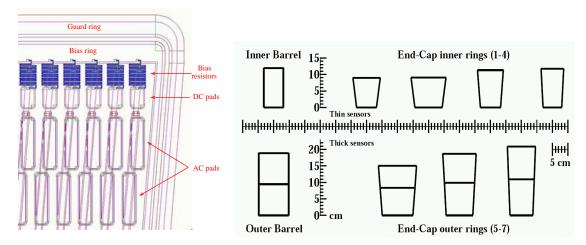
Figure 48: Left panel: Drawing of one corner of the active region of a wedge-shaped silicon strip sensor for the tracker endcaps. Right panel: Silicon sensor geometries in the CMS tracker.
