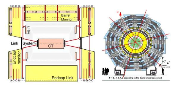
Figure 218: Schematic view of the alignment system. Left panel: longitudinal view of CMS. The continuous and dotted lines show different optical light paths. Right panel: transverse view of the barrel muon detector. The crossing lines indicate the r-z alignment planes with  $60^{\circ}$  staggering in  $\phi$ .
