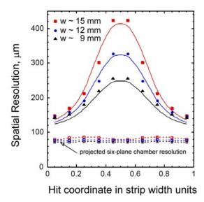
Figure 196: Left panel: ME1/1 chamber single-plane resolution vs. HV. Right panel: Ultimate large CSC offline resolutions per plane for different muon passage points across a strip for areas with different strip widths for data (closed symbols) and simulation (solid lines). The expected overall 6-plane CSC resolutions are shown by open symbols and dashed lines.
