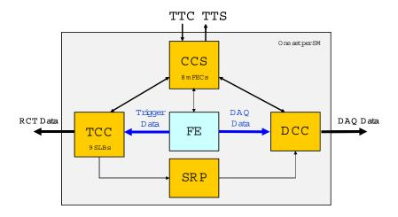
Figure 80: Schematic view of ECAL off-detector electronics.
