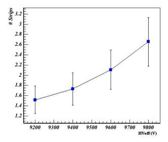
Figure 213: Profile histogram of the chambers' cluster-size distribution as a function of  $HV_{\rm eff}$ . The dots and bars are the average and the root-mean-square of the cluster-size distributions, respectively.
