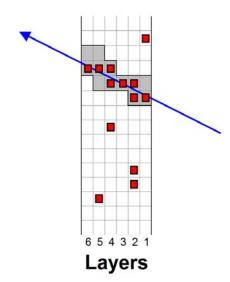
Figure 187: Left panel: muon signals as seen at the AFEB amplifier output. Right panel: a schematic event display showing anode signals in the 6 planes of a CSC (small dark squares). The ALCT board FPGA logic is programmed to scan the chamber and search for hits falling inside predefined patterns (grey cells) consistent with muons originating from the interaction point. Hits must be present in at least 4 planes for an ALCT pattern to be found.
