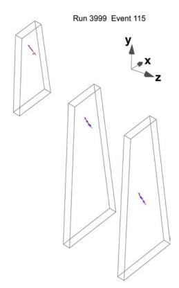
Figure 190: Part of a CMS event display showing a muon event detected by CSCs during the MTCC. Only those chambers containing muon hits are displayed.
