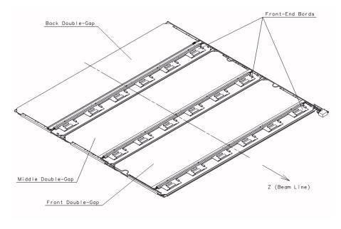
Figure 201: Schematic layout of chamber module with 3 double-gaps.
