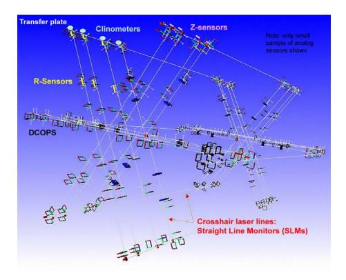
Figure 221: Visualisation of the geometry and components of the muon endcap alignment system. The square objects represent optical sensors (DCOPS) for monitoring 3 straight laser lines across each endcap station.
