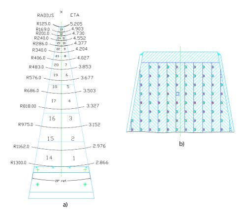
Figure 120: a) Transverse segmentation of the HF towers. b) An expanded view of the wedge shows the squared out groove holding the radioactive source tube.
