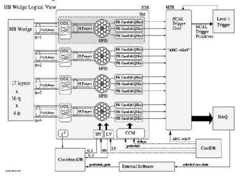
Figure 122: Overview of HCAL read-out/trigger chain and connections to database.
