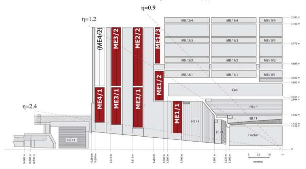
Figure 179: Quarter-view of the CMS detector. Cathode strip chambers of the Endcap Muon system are high-lighted.
