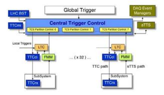
Figure 234: Trigger Control System architecture.
