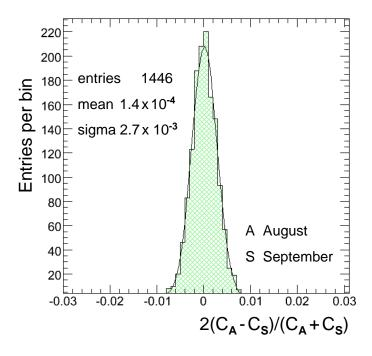
Figure 82: Distribution of differences of inter-calibration coefficients from a supermodule exposed to a high energy electron beam on two occasions, separated by a period of one month. The reproducibility of the intercalibration coefficients (RMS/ $\sqrt{2}$ ) is measured to be 0.2%.
