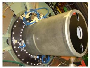
Figure 223: Left panel: Link Disk and Alignment Ring installed in the inner  $\eta = 3$  cone during the first closing of the detector in summer 2006, MTCC period. Right panel: Alignment Ring mounted in the TEC end flange.
