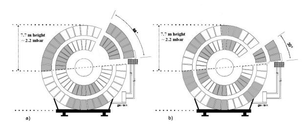
Figure 209: In each endcap disk the RPC detectors are divided in 2 rings. RE1 (a) is divided into 60° sectors, while in RE2 and in RE3 (b) sectors are composed of 3 chambers of the internal ring and the corresponding 3 of the external ring. Every sector is supplied by 2 independent gas lines.
