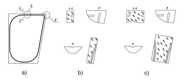
Figure 105: a) Basic structure of a scintillator tile with a groove to fix wavelength shifting fibre, b) cross section of the 3.7-mm-thick scintillator for layers 1-17, and c) cross section of the 9-mm-thick scintillator for layer zero. Two layers of reflecting paint cover the side surfaces of the tile.
