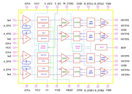
Figure 146: Block diagram of the MAD ASIC.
