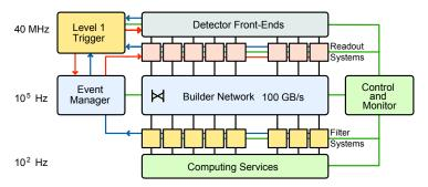
Figure 235: Architecture of the CMS DAQ system.
