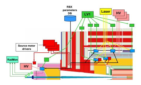
Figure 123: Overview of HCAL detector controls.
