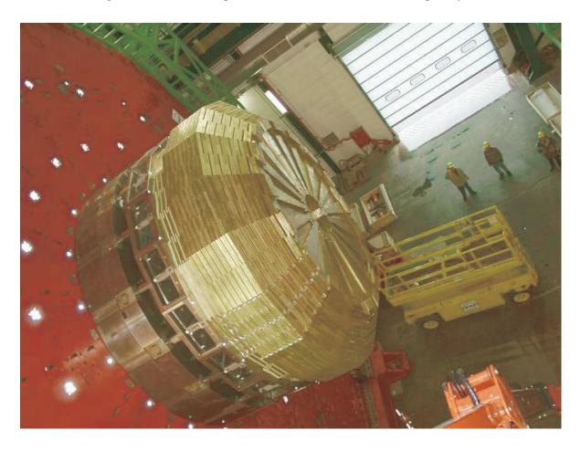
Figure 103: Partially assembled HE-minus absorber in the CMS surface hall (SX5). Scintillator trays can be seen to be inserted in some of the outer sectors.
