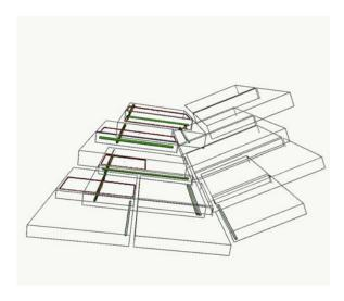
Figure 214: Iguana muon reconstruction: RPC-fired strips are in red and DT hits in green.
