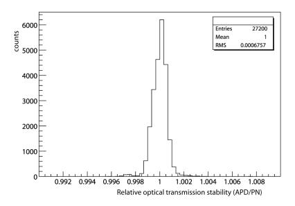
Figure 88: Stability of crystal transmission measurements at 440 nm (blue laser) over 11.5 days operation for a module of 200 crystals.
