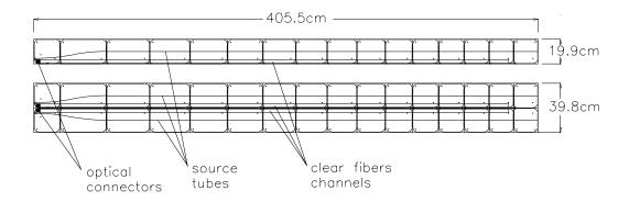
Figure 96: Scintillator trays.
