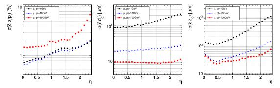
Figure 33: Resolution of several track parameters for single muons with transverse momenta of 1, 10 and 100 GeV: transverse momentum (left panel), transverse impact parameter (middle panel), and longitudinal impact parameter (right panel).
