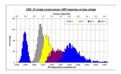
Figure 255: MIP response of BCM1F single-crystal diamond with front-end electronics, as a function of bias voltage of the sensor. The superposition of histograms around 0-V output amplitude indicates the noise.
