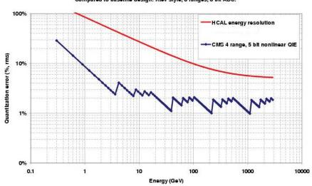
Figure 124: Contribution of the FADC quantization error to the resolution, compared with a representative HCAL resolution curve.
