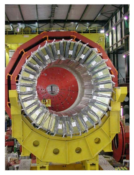
Figure 93: Assembled HCAL half-barrel in SX5, the above ground assembly hall.
