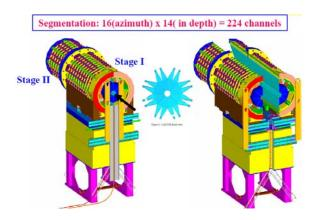
Figure 129: CASTOR calorimeter and support.
