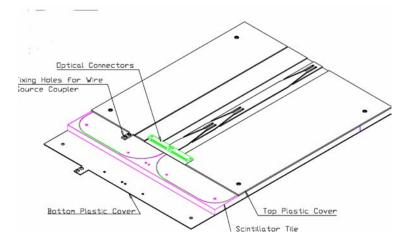
Figure 117: The arrangement of scintillation tiles, plastic covers and connectors in a tray. The components are slightly displaced from their true positions to show their matching designs.
