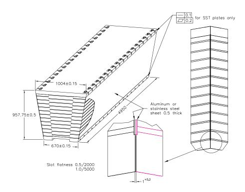
Figure 95: Isometric view of the HB wedges, showing the hermetic design of the scintillator sampling.
