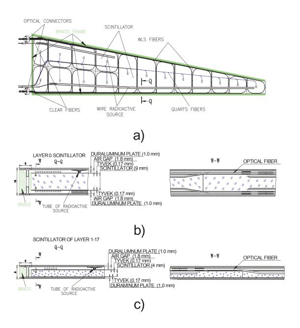
Figure 106: The design of the calorimeter scintillator trays: a) front view of a tray without upper aluminium cover, b) cut out view of the layer-0 tray with two fibres from a tile, c) cut out view of a tray for layers 1–17.
