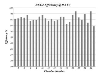
Figure 211: Efficiency at HV = 9.3 kV for the first 27 endcap chambers.
