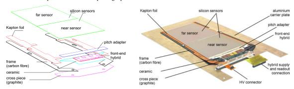
Figure 51: Left panel: Exploded view of a module housing two sensors. Right panel: Photograph of a TEC ring 6 module, mounted on a carrier plate.
