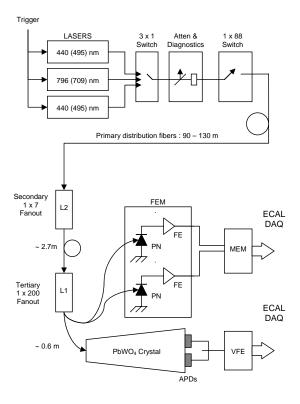
Figure 86: The components of the laser monitoring system.
