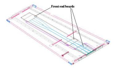
Figure 204: A view of an endcap RPC chamber.
