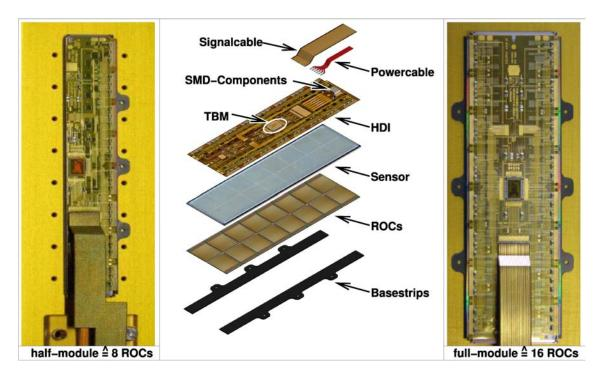
Figure 42: Exploded view (middle panel) of a barrel pixel detector full module (right panel) and picture of an assembled half module (left panel).
