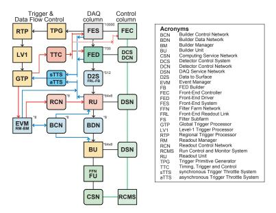
Figure 236: Schematic of the functional decomposition of the DAQ. The multiplicity of each entity is not shown for clarity.
