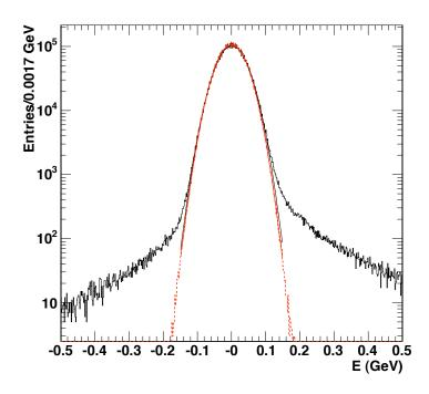
Figure 90: Reconstructed amplitude in ECAL barrel channels in the absence of a signal, without pileup (dashed histogram) and with pileup (solid histogram). A Gaussian of width 40 MeV is superimposed on the dashed histogram.
