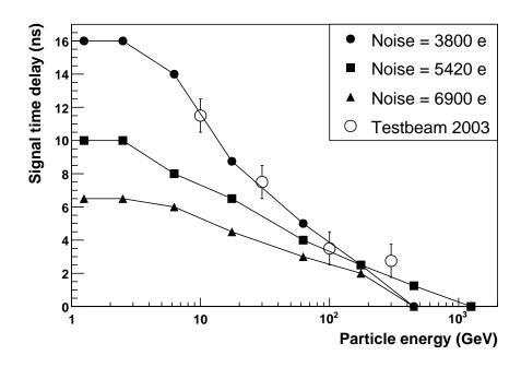
Figure 127: Pulse time variation as a function of signal amplitude as measured on the bench (solid points) for several input amplifier configurations compared with test beam measurements from 2003.
