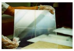
Figure 115: View of a typical tile of HO with WLS fibres inserted in the 4 grooves of the tile.
