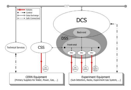
Figure 253: Context diagram of the DSS system, showing its rôle with respect to the CERN Safety System (CSS), the Detector Control System (DCS) and other technical services. The interconnection network is provided by the Data Interchange Protocol (DIP).
