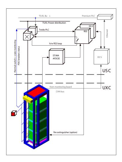
Figure 250: Control loops for rack powering.
