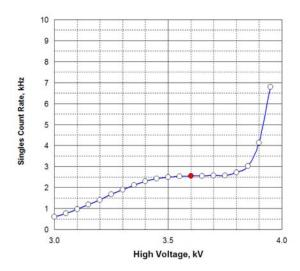
Figure 184: Left panel: CSC gas gain vs. high voltage. Right panel: ME2/1 chamber singles rate vs. high voltage (the overall sensitive area of all 6 planes in this chamber is  $\approx 9.5$  m<sup>2</sup>).
