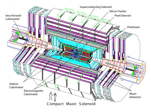
Figure 1: A perspective view of the CMS detector.
