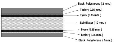
Figure 116: Cross section of a HO tray showing the different components.
