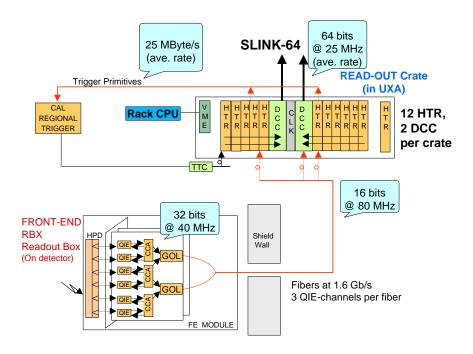
Figure 121: Overview of HCAL read-out electronics.
