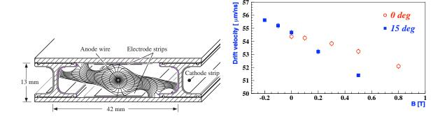
Figure 165: Simulation of the distortion produced in the drift lines by a 0.5 T magnetic field parallel to the wires.
