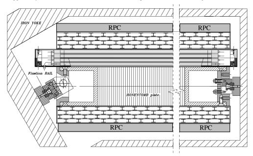
Figure 136: A DT chamber in position inside the iron yoke; the view is in the  $(r-\phi)$  plane. One can see the 2 SLs with wires along the beam direction and the other perpendicular to it. In between is a honeycomb plate with supports attached to the iron yoke. Not shown are the RPCs, which are attached to the DT chambers via support plates glued to the bottom and/or top faces, depending on chamber type.
