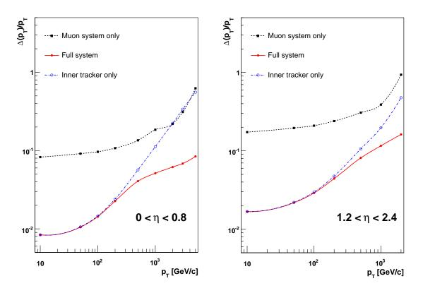
Figure 2: The muon momentum resolution as a function of the momentum  $(p_T)$  using the muon system only, the inner tracking only, and both. Left panel:  $|\eta| < 0.8$ , right panel:  $1.2 < |\eta| < 2.4$ .
