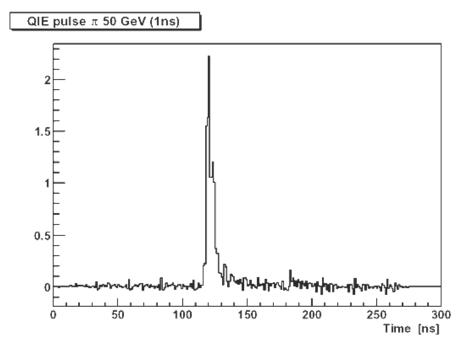
Figure 126: Measured pulse shape, energy collected vs. time, for HF.
