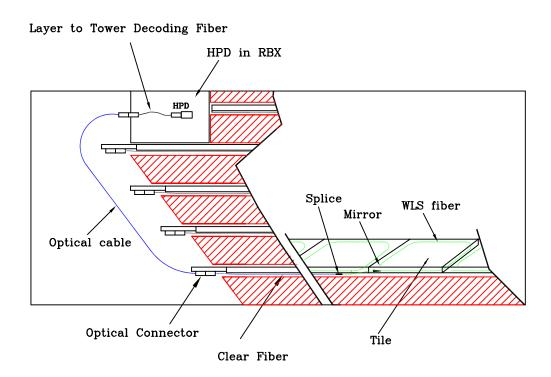
Figure 98: Schematic of the HB optics.
