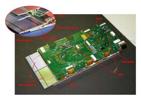
Figure 81: Photograph of a complete type-1 ladder, with an inset showing details of a micromodule
