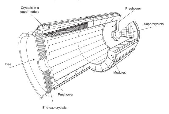
Figure 75: Layout of the CMS electromagnetic calorimeter showing the arrangement of crystal modules, supermodules and endcaps, with the preshower in front.
