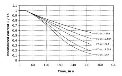
Figure 24: The normalised discharge current as a function of time for different initial currents, showing the effect of the increase in magnet and external dump resistance with current.
