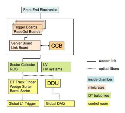
Figure 145: Block diagram of the DT electronic system.
