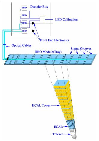
Figure 111: Schematic view of a HO tray shown with individual tiles and the corresponding grooves for WLS fibres. Each optically independent (4 WLS fibres) tile is mapped to a tower of HB. Optical fibres from the tray are routed to the decoder box which contains the photodetector and read-out electronics.
