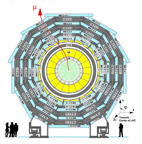
Figure 135: Layout of the CMS barrel muon DT chambers in one of the 5 wheels. The chambers in each wheel are identical with the exception of wheels –1 and +1 where the presence of cryogenic chimneys for the magnet shortens the chambers in 2 sectors. Note that in sectors 4 (top) and 10 (bottom) the MB4 chambers are cut in half to simplify the mechanical assembly and the global chamber layout.
