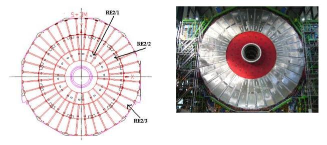
Figure 202: Left panel: Schematic r- $\phi$  layout of RPC station RE2 on the back side of the first endcap yoke. Right panel: RPC station RE2 on the back side of the YE-1 yoke. The inner ring has been staged and is absent here.
