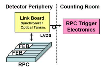
Figure 205: Block diagram of RPC read-out electronics.
