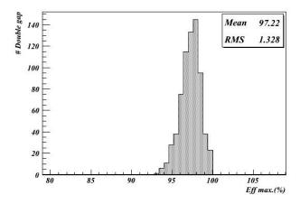
Figure 210: Distribution of plateau efficiency for all the barrel chambers.
