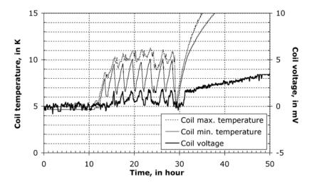
Figure 28: The minimum and maximum temperatures and voltage of the coil as a function of time, with only a few amperes of current, showing the superconducting-to-resistive-state transition at around  $9.3~\mathrm{K}$ .
