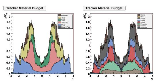
Figure 32: Material budget in units of radiation length as a function of pseudorapidity  $\eta$  for the different subdetectors (left panel) and broken down into the functional contributions (right panel).
