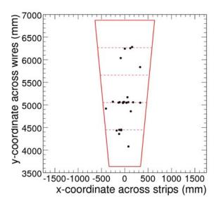
Figure 191: Left panel: single-plane anode signal efficiency (open circles) and ALCT pattern finding efficiency (filled circles) vs. high voltage. Right panel: predicted position of muon tracks in ME2/2 chambers for events when no LCT was found in these chambers (superimposed results for 6 chambers). The dashed lines indicate where wire planes of the ME2/2 chambers have inefficient bands separating independent HV segments.
