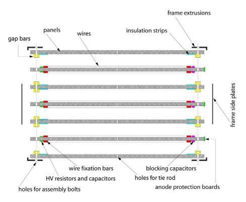
Figure 183: Mechanical design of the CMS cathode strip chambers (exploded view).
