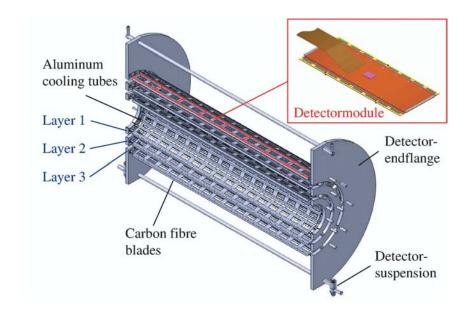
Figure 40: Complete support structure half shell with the three detector layers.
