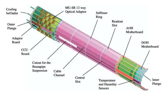
Figure 41: Overview of a supply tube half shell.
