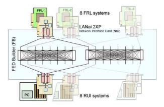
Figure 243: 8×8 FED builder with a two-rail network.
