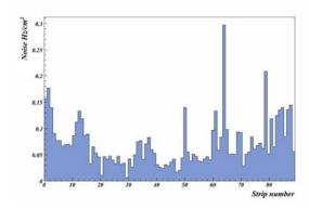
Figure 215: Barrel chamber noise profile at  $HV_{eff} = 9.6 \text{ kV}$ .
