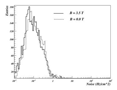
Figure 216: Noise distributions in 2 different magnetic fields. All strips of the barrel stations are included in the distribution.
