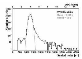
Figure 68: Normalized common mode subtracted single strip noise for TIB (left panel) and TID (right panel), in deconvolution mode. Details are described in the text.
