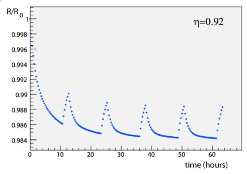
Figure 84: Simulation of crystal transparency evolution at LHC based on test-beam results. For this illustrative example a luminosity of  $\mathcal{L}=2\times10^{33}~\text{cm}^{-2}\text{s}^{-1}$  was assumed, together with a machine cycle consisting of a 10 hour coast followed by 2 hours filling time. The crystal behaviour under irradiation was modeled on data taken during a crystal irradiation in the test beam.
