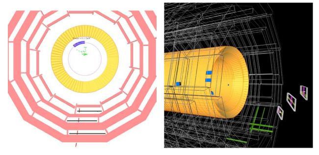
Figure 176: Event displays from the MTCC. Left panel: muon reconstructed in a DT sector in conjunction with Tracker activity. Right panel: muon track passing through both DT and CSC chambers.
