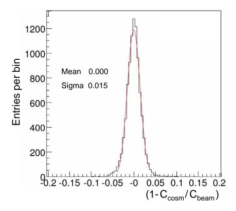
Figure 83: Distribution of the relative differences between the inter-calibration coefficients measured with high energy electrons and those obtained from cosmic ray muons.
