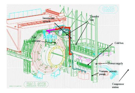
Figure 12: The layout for the surface test at SX5, showing only the central barrel. The magnet is connected to the cryoplant (through the proximity cryogenics), the vacuum and the power systems.
