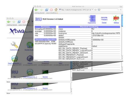
Figure 247: Example HyperDAQ page. Clicking on the RU application in the HyperDAQ page brings up monitoring information for the Read-out Unit application.
