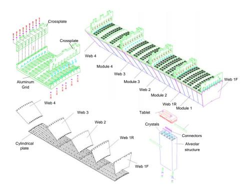
Figure 73: Layout of the ECAL barrel mechanics.
