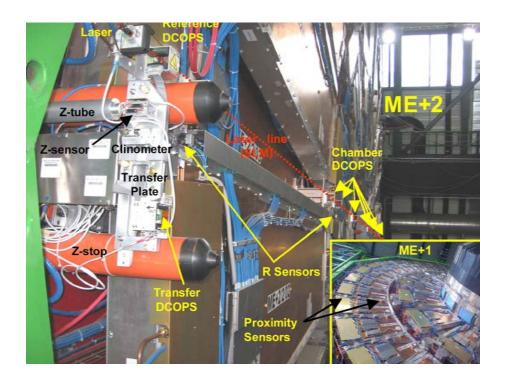
Figure 222: Close-up of one of the 3 Straight Line Monitors (SLM) on the ME+2 station with cross-hair laser, DCOPS, and analog sensors (r, z, and Tiltmeter). The insert indicates the location of proximity sensors on ME+1.
