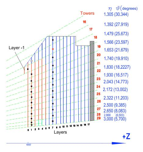
Figure 109: Longitudinal and angular segmentation of the HE calorimeter. The dashed lines point to the interaction point.
