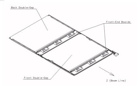
Figure 200: Schematic layout of chamber module with 2 double-gaps.
