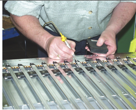
Dispensing normal (left) and conductive (right) glue.
