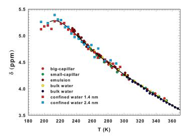
Fig. 41. – The proton chemical shift of water,  $\delta$ , as a function of temperature. Literature data are plotted as circles and the present data are plotted as squares symbols. The line is a guide for the eye.
