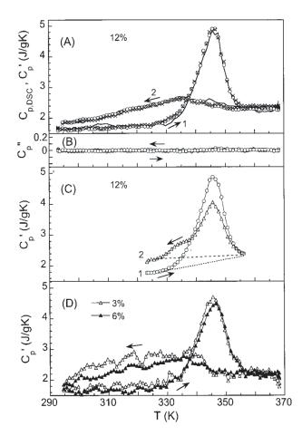
Fig. 31. – The specific heat measured in glycerol. The maximum gives clear indication of the onset of the glass transition.
