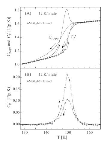
Fig. 30. – The real and imaginary parts of the specific heat measured during the cooling and heating at a rate of 12 K/h [274].
