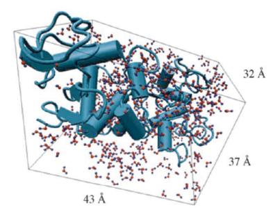
Fig. 59. – Snapshot from a MD simulation at T = 250K and P = 1atm of the hydrated lysozyme powder model, containing two protein molecules and 484 water molecules around them (hydration level h = 0.3).
