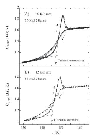
Fig. 29. – The specific heat measured in 5-Methyl-2-Hexanol in two different thermal rates (60K/h and 12K/h). The thermal cycle procedure used is represented in the figure by the arrows: the sample has first been cooled and afterwards heated [274].
