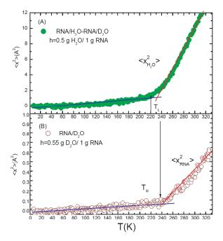
Fig. 52. – The slope of the MSD vs T curve used as a measure of the biomaterial softness. This figure shows the case of RNA and its hydration water. As one can see, above the crossover temperature  $(T_C)$ , the RNA becomes 15 times softer than its glassy state, while the hydration water becomes 20 times softer when crossing the temperature  $T_L$ .
