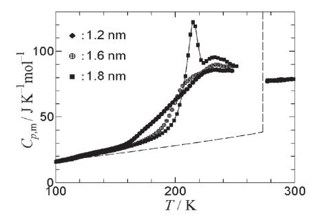
Fig. 38. – The molar heat capacity  $C_{p,m}$  measured in water confined in silica nanotubes (MCM-41 samples with a pore diameter of 1.2, 1.6 and 1.8nm). The results are compared with specific heat data of ice and bulk water  $(T \ge 270K)$  [300].
