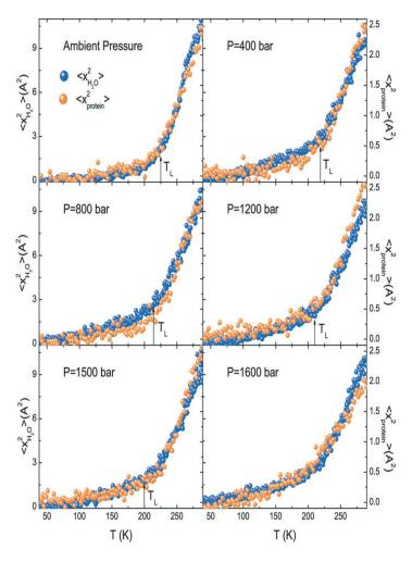
Fig. 54. – Reduced plot of pressure dependence of MSD of protein and its hydration water. It is to be noted in this figure that the crossover temperature of the protein and its hydration water is closely synchronized at a range of pressures below 2000 bar.
