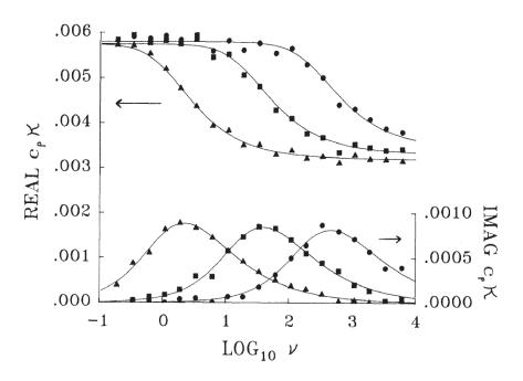
Fig. 28. – The real and imaginary part of the specific heat,  $C_p \kappa$ , measured in propylene glycol as a function of the temperature [271].
