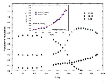
Fig. 24. – The FWHM values of the OH stretching spectral component I ( $3120cm^{-1}$ ) vs. T, measured in confined water and in the LDA phase [199, 226] (inset). Temperature dependence of the fractioned relative populations of the LDL,  $W_{LDL}$ , (diamonds) and of the HDL,  $W_{HDL}$ , (triangles and circles) water phases. For the HDL phase, NHB (circles) and PHB (triangles) contributions are reported separately (ref. [244]).
