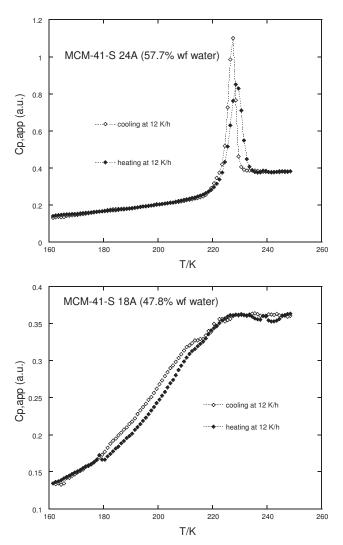
Fig. 40. – The specific heat  $C_{p,app}$  in water confined in MCM-41-S sample with a diameter of 2.4nm (upper figure) and 1.8nm (down figure) measured by using a modulated calorimeter. In both the experiments the heating and cooling rate is of 12K/h [306].
