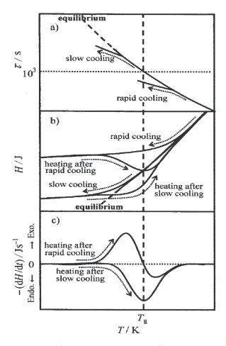
Fig. 34. – Relationship between a) the relaxation time  $\tau$ , b) the enthalpy H, and c) the spontaneous enthalpy-relaxation rate -dH/dt as a function of T, observed in the dynamical arrest region with a single characteristic time for the molecular rearrangement.  $T_g$  was determined empirically as the point at which the rapidly cooled sample showed a change (against temperature) in dH/dt from positive to negative and the slowly cooled sample showed a minimum dH/dt value [295].
