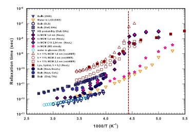
Fig. 76. – The figure, in a log -lin plot, shows in an enlarged scale the same data ( $\tau$  vs. 1000/T) reported in the previous one (Fig. 75). In addition, neutron scattering data obtained in bulk (incoherent [394] ad coherent [420]) and in hydrated lysozyme with h = 0.3 [201] are reported.
