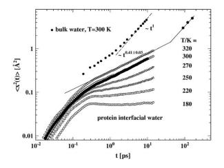
Fig. 78. – The figure reports the time-resolved mean square displacement  $(\langle x^2(t) \rangle$  vs. t) of bulk water and of myoglobin hydration water (h = 0.4) measured by using neutron scattering [421]. Each curve corresponds to a different temperature in the range 180 < T < 320K.
