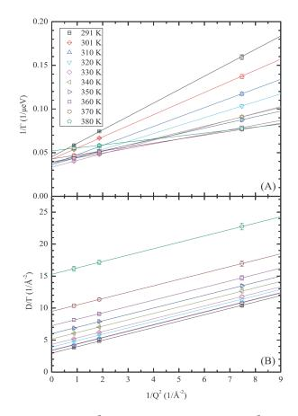
Fig. 69. – The plots of  $1/\Gamma$  vs  $1/Q^2$  (panel A) and of  $D/\Gamma$  vs  $1/Q^2$  (panel B) for measured temperatures from 291 to 380K at low  $Q = 0.37, 0.73, 1.07 \text{ }^{A^{-1}}$ . The solid lines are the fitting results. The slopes of the straight lines in panel A give the inverse diffusion constant 1/D, whereas the zero intercepts in panel B give  $\xi^2$ .
