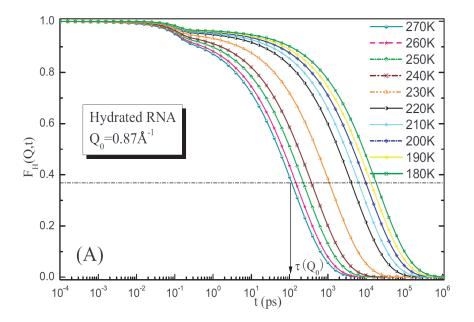
Fig. 49. – Intermediate scattering functions ISF at  $Q_0$  of hydrogen atoms in RNA hydration water, as a function of temperature. They are extracted from analysis of the quasielastic spectra by using the relaxing-cage model. It is seen that the ISF exhibits a two-step decay consisting of the beta and the alpha relaxation processes.
