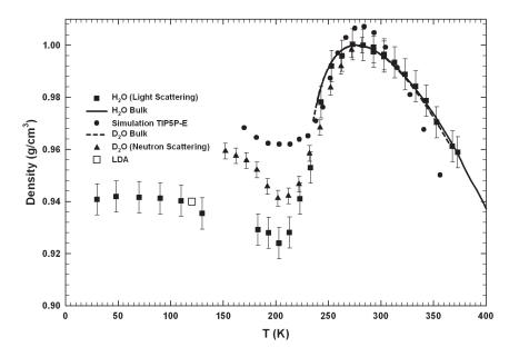
Fig. 25. – The measured  $\rho_{H_2O}(T)$  vs. T (squares, ref. [244]); the solid and dot lines refer to bulk densities of  $H_2O$  and  $D_2O$ , respectively [239-241]. Triangles represent the  $\rho_{D_2O}(T)$  measured by means of neutron scattering [97]. Dots are the bulk density values calculated by the MD simulation [77]. The open square represents the density of the LDA water at T = 120K [238]. Heavy water densities are properly scaled over the  $\rho_{H_2O}$  ones.
