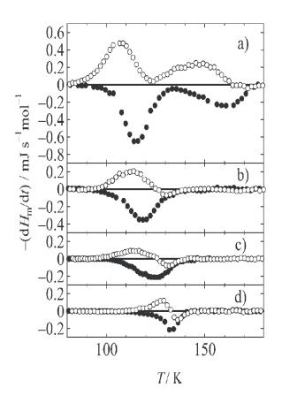
Fig. 35. – Heat capacities of mixtures of water and ice confined in silica gel of a) 1.1 - nm, b) 6 - nm, c) 12 - nm, and d) 52 - nm average pore diameter [293]. Lines represent the literature results of bulk water and ice [299], and filled circles a) represent the data obtained for the sample cooled to 235K and measured in the heating direction.
