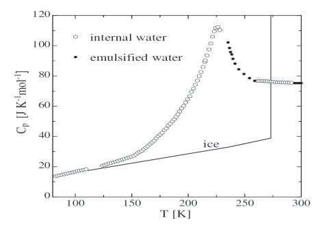
Fig. 39. – Heat capacity of internal, emulsified water and ice [31] [300].
