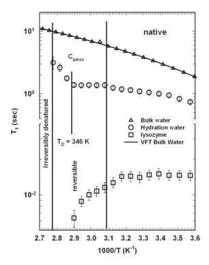
Fig. 47. – The temperature evolution of the NMR longitudinal spin-lattice relaxation time  $T_1$  for temperatures above and below the region of protein denaturation. Triangles correspond to bulk water, circles to protein hydration water, and squares to protons in the protein. The dramatic changes in  $T_1$  further demonstrate the role played by hydration water in the denaturation process [317].
