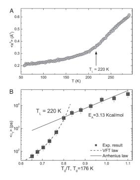
Fig. 44. – Evidence for the dynamic transition in lysozyme. (A) The temperature dependence of the mean-squared atomic displacement of the hydrogen atom at 2 ns time scale measured by an elastic scan with resolution of 0.8eV. (B) Temperature dependence of the average translational relaxation times plotted in log(T) vs.  $T_0/T$ , where  $T_0$  is the ideal glass transition temperature [201].
