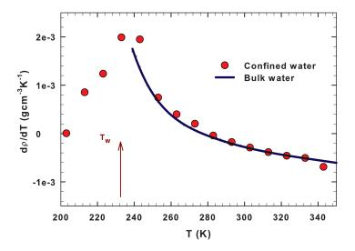
Fig. 26. – The derivative of the density with respect to temperature  $(\partial \rho / \partial T)_P$ . As it can be observed such a quantity is characterized by a maximum just at the Widom temperature  $T_W$ , indicated by the arrow.  $(\partial \rho / \partial T)_P$ , related with the cross-correlation between the entropy and volume fluctuations, is proportional to the thermal expansion coefficient.
