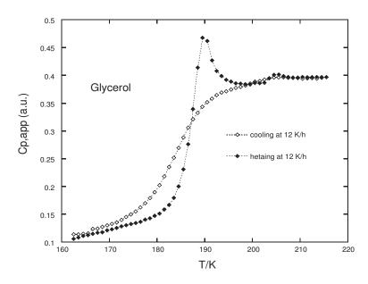
Fig. 27. – The specific heat measured in Glycerol. The maximum gives the clear indication of the onset of the glass transition.
