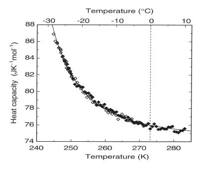
Fig. 33. – Heat capacity of bulk water measured as a function of temperature. Different symbols deal with the two studied samples; the full line is the curve fitting the experimental points [281].
