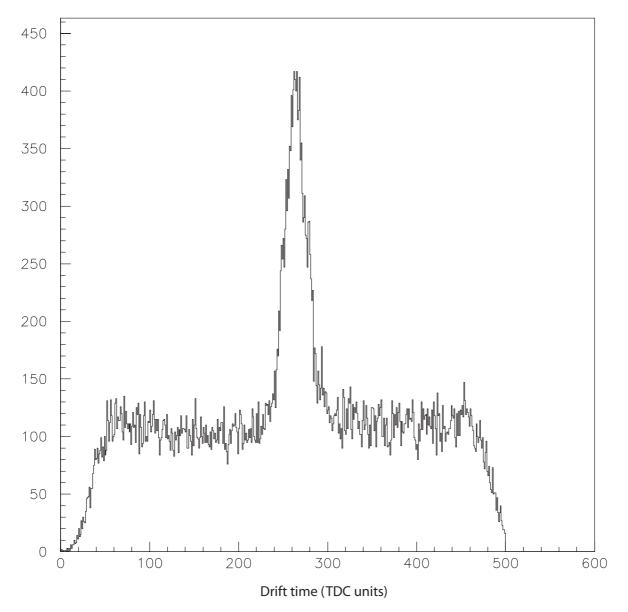
Figure 2- Drift-time distribution for vertical cosmics. Conditions and selections as in Figure 1
