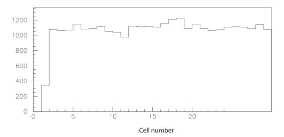
Figure 3- Occupancy of the first half of the layer 2 of SL 2 for verical cosmic. The second half is not shown since HV was disconnected.
