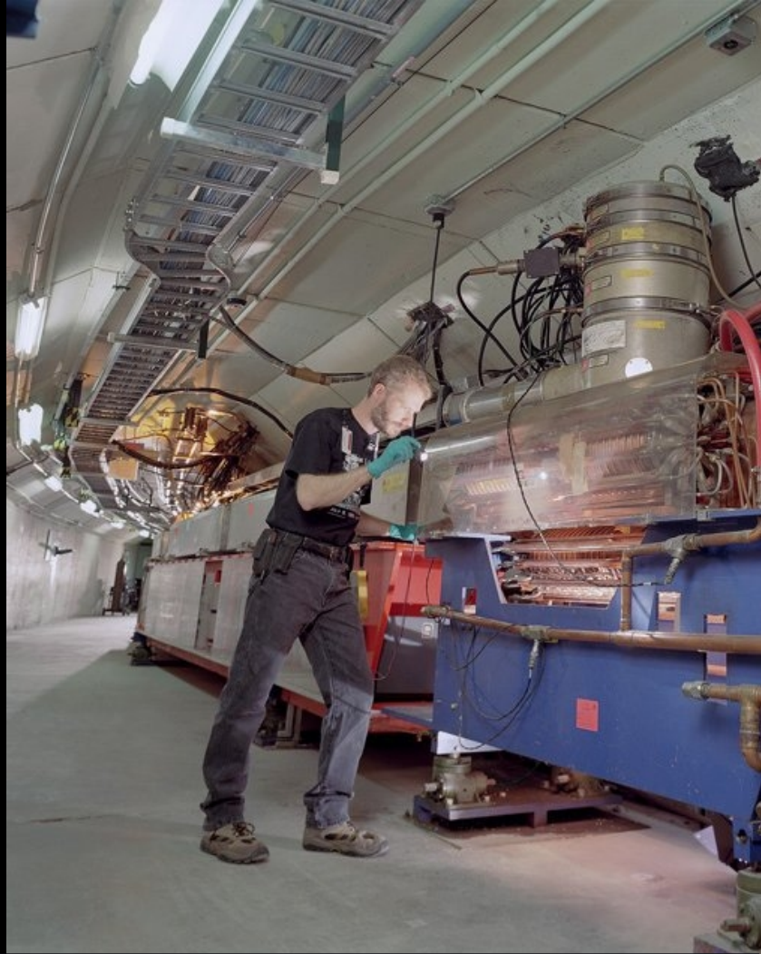
The Booster synchrotron strips electrons off H^- and accelerates remaining protons up to 8 GeV
