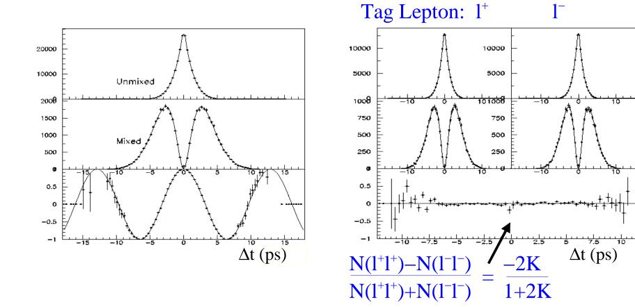
•Using true  $\Delta t$ :  $\tau_{B0} = 1.533 \pm 0.003 \text{ ps}$   $\Delta m_{d} = 0.488 \pm 0.001 \text{ ps}^{-1}$ K = -0.001 \pm 0.002 •Using true  $\Delta z$ :  $\tau_{B0} = 1.539 \pm 0.003 \text{ ps}$   $\Delta m_{d} = 0.483 \pm 0.001 \text{ ps}^{-1}$ K = -0.001 \pm 0.002
