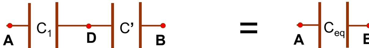
$$C_{eq} = \left[ \frac{1}{C_1} + \frac{1}{C_2} \right]^{-1} = 1.5 \text{ nF}$$
